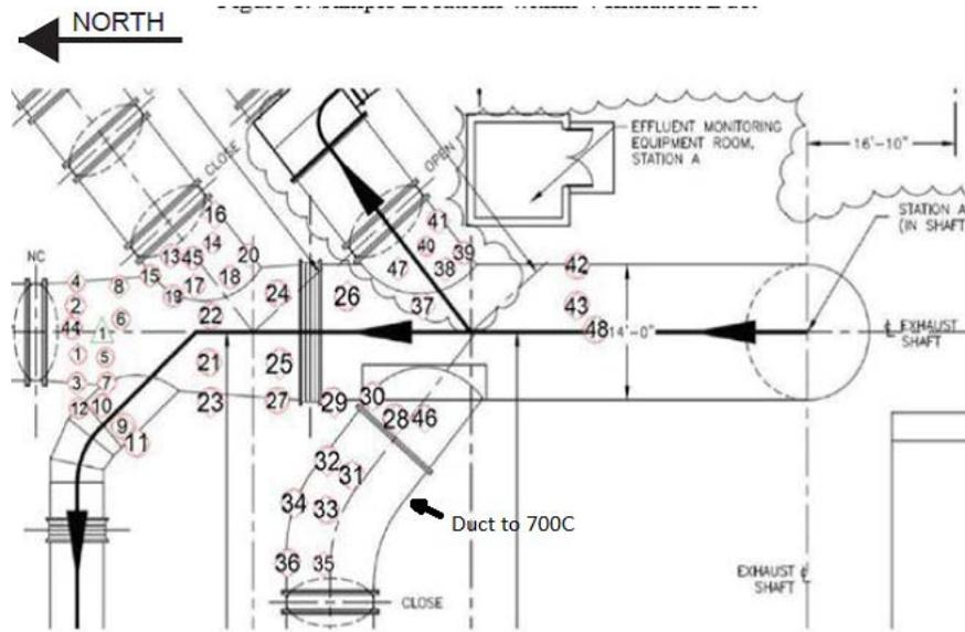
Figure 10 - Sample Locations within Ventilation Duct
