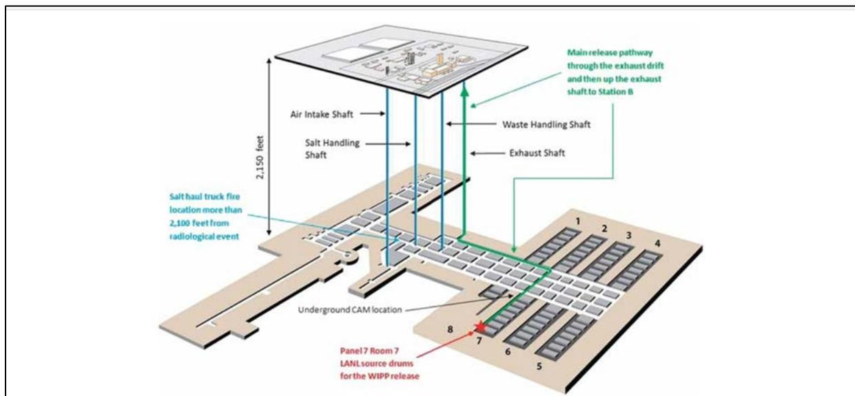
Figure 1 - WIPP Facility Configuration
