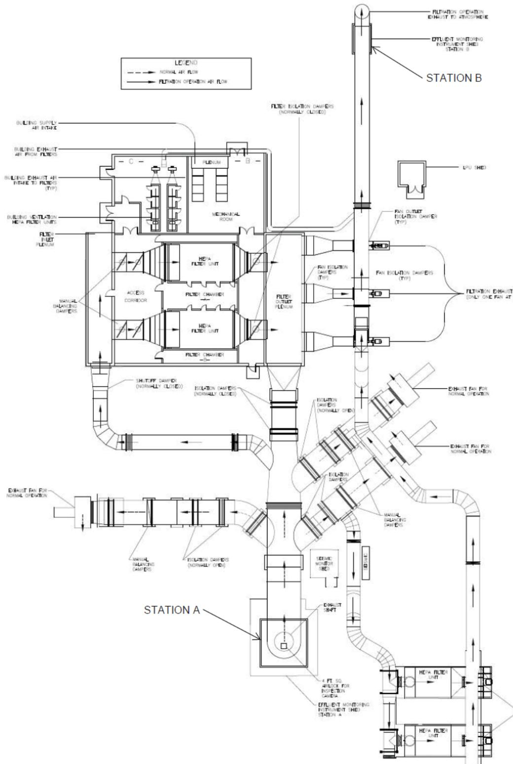
Figure 4 - Underground Ventilation System with IVS
