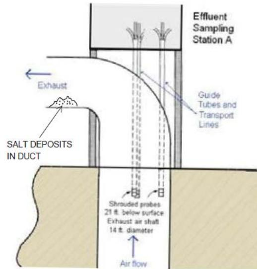
Figure 8 - Effluent Sample Station A
