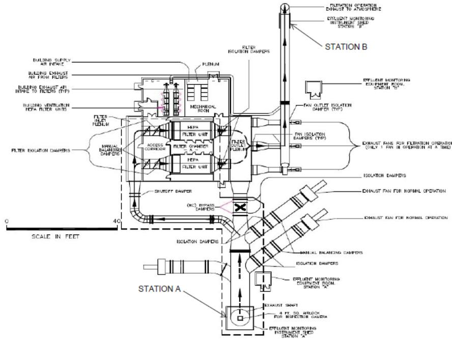
Figure 2 - 2014 UVS System Layout
