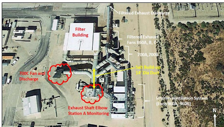
Figure 6 - Labeled Above Ground Image of the Ventilation System
