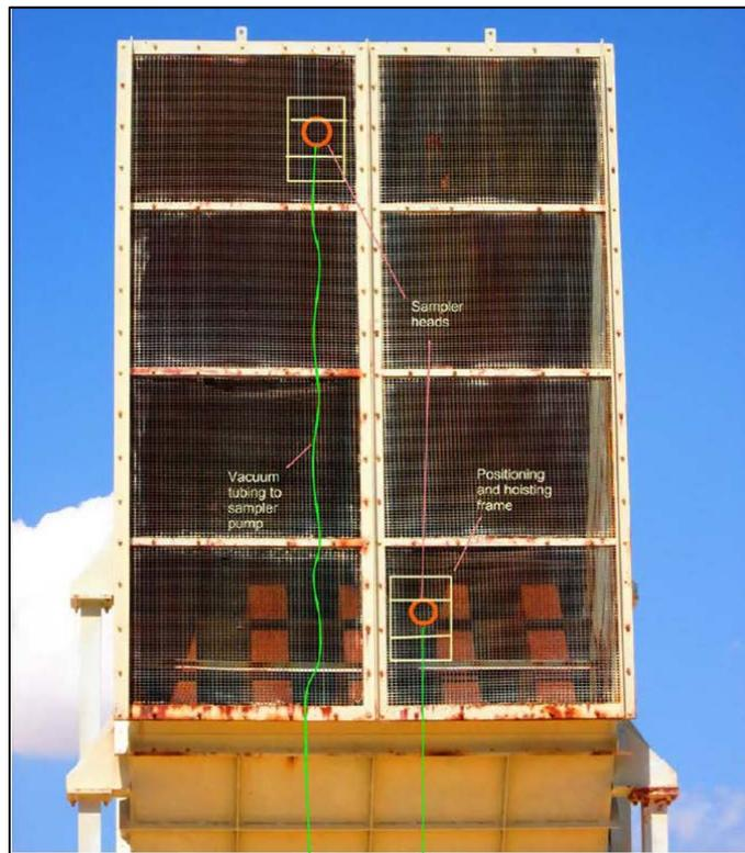
Figure 11 - Air Sampling on Face of 700C Fan
