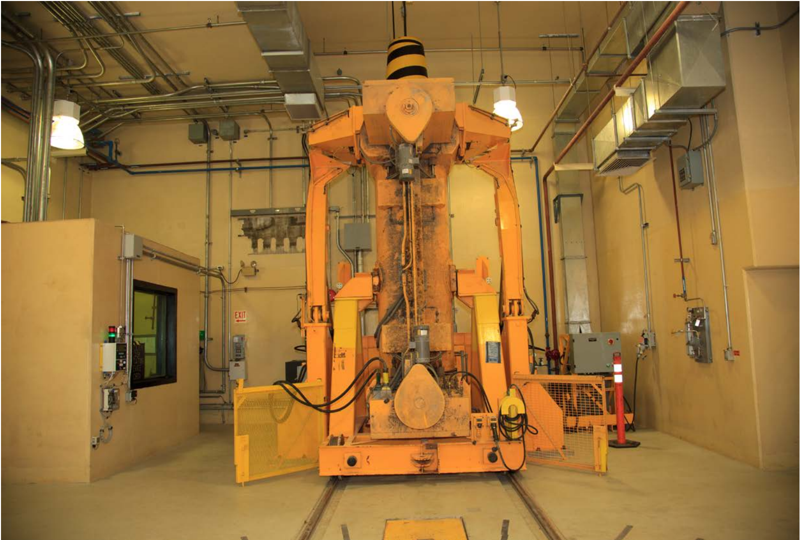
Figure 4-11 Facility Cask Loading Room and Facility Cask Rotating Device
