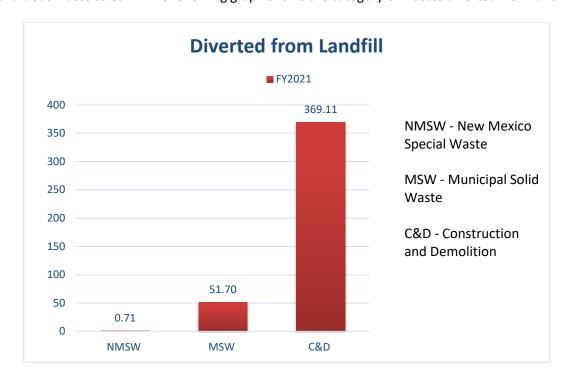
The C&D diversion is high largely due to the 369 metric tons of recycled mixed metal from the General Plant Projects (GPP) new construction excess building material scrap from across the site to include the Site Significant Containment Ventilation System (SSCVS) and new Utility Shaft projects.
