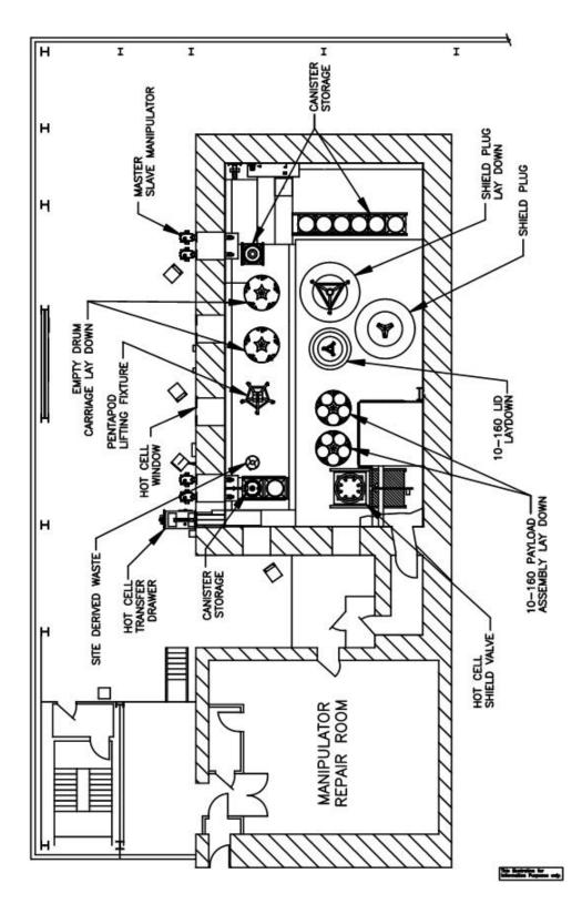
Figure A1-17b RH Hot Cell Storage Area
