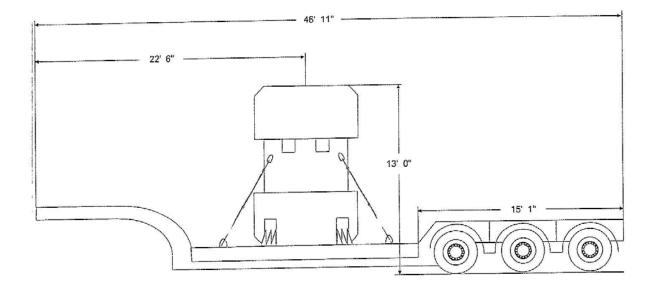
Figure A1-19 CNS 10-160B Shipping Cask on Trailer
