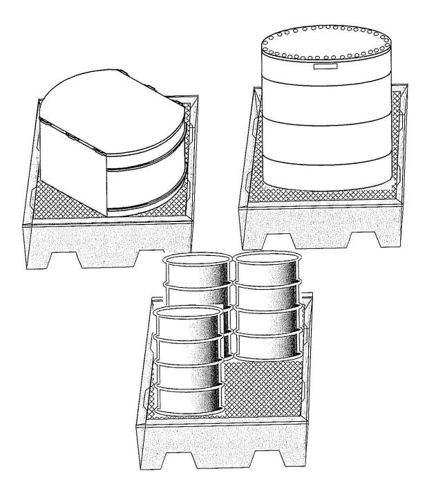
Figure A1-10a Typical Containment Pallet
