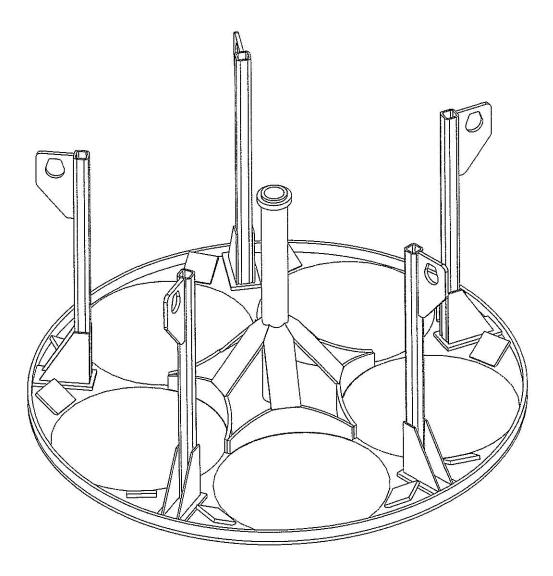
Figure A1-25 CNS 10-160B Drum Carriage
