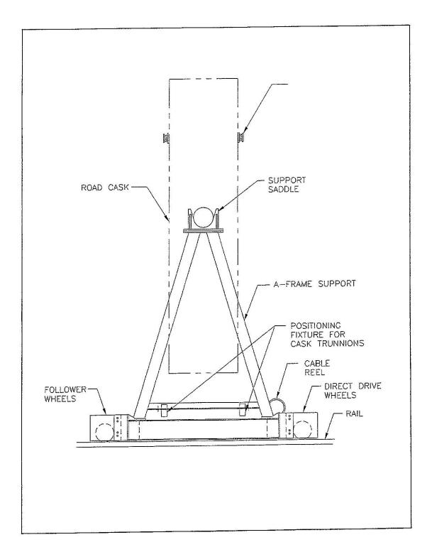
Figure A1-22a RH-TRU 72-B Cask Transfer Car
