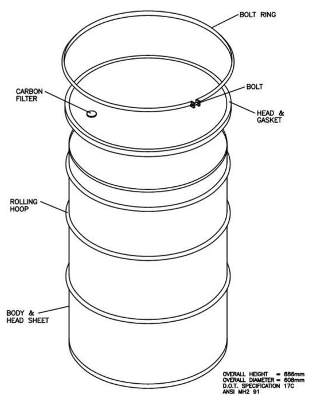
Figure A1-3 Standard 55-Gallon Drum (Typical)
