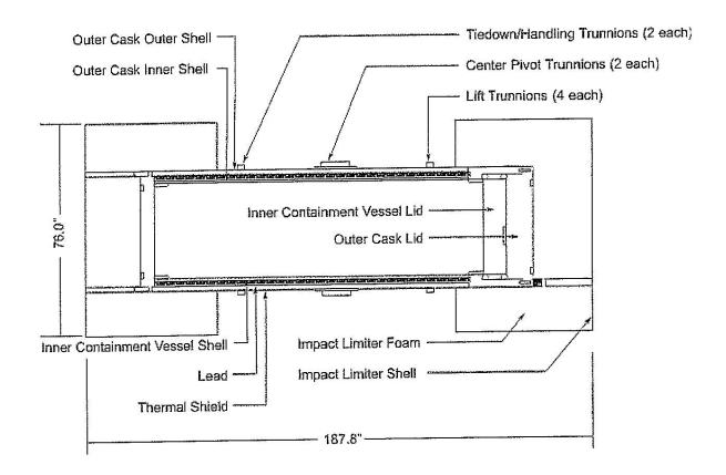
Figure A1-20 RH-TRU 72-B Shipping Cask for RH Transuranic Waste (Schematic)
