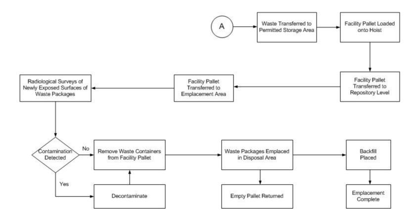
Figure A1-13 WIPP Facility Surface and Underground CH Transuranic Mixed Waste Process Flow Diagram (Continued)
