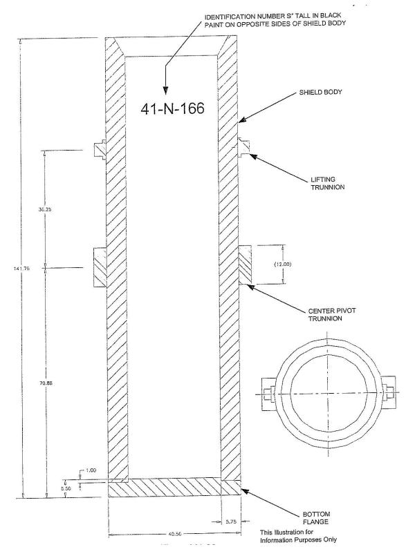
Figure A1-30 RH Shielded Insert Assembly
