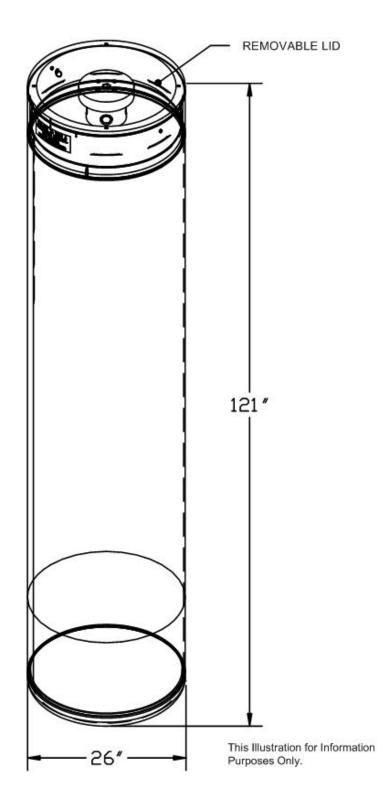
Figure A1-16a RH-TRU 72-B Canister Assembly
