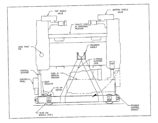
Figure A1-24 RH Facility Cask Transfer Car (Side View)
