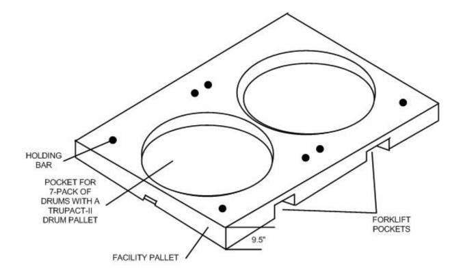
Figure A1-10 Facility Pallet for Seven-Pack of Drums
