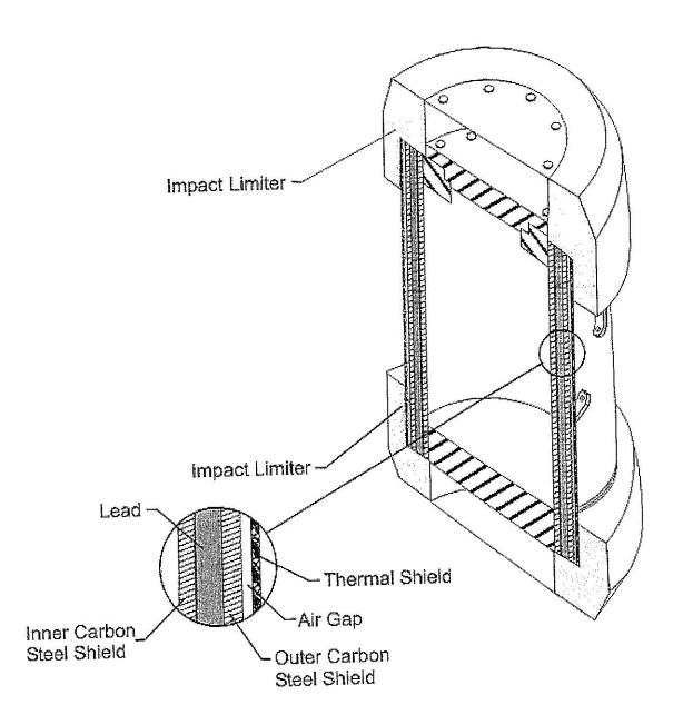
Figure A1-21 CNS 10-160B Shipping Cask for RH Transuranic Waste (Schematic)
