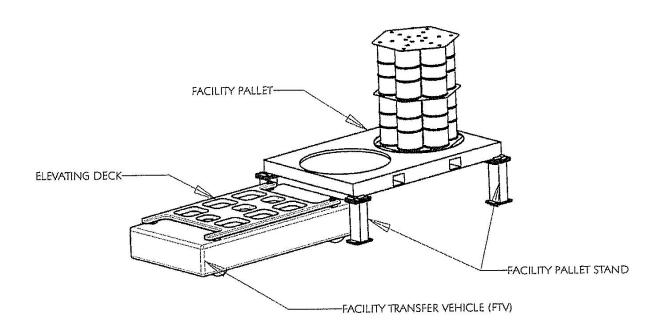
Figure A1-11 Facility Transfer Vehicle, Facility Pallet, and Typical Pallet Stand
