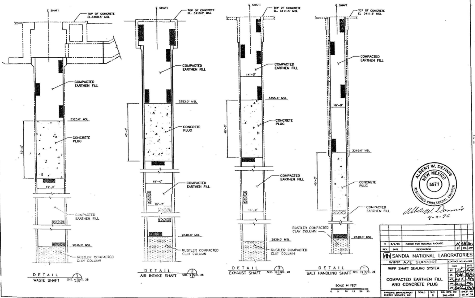
Compacted Earthen Fill and Concrete Plug
