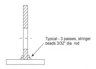
Figure 2.3-3 – Weld-On Lifting Lug Detail
