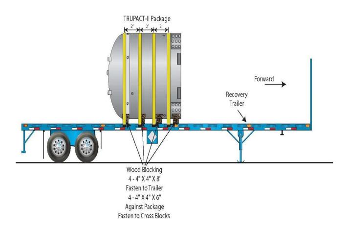
Figure 2.3-10 – Horizontal Package Transport Securement
