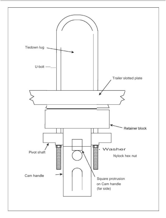
Figure 2.3-8 — Complete Cam Handle Tiedown Assembly
