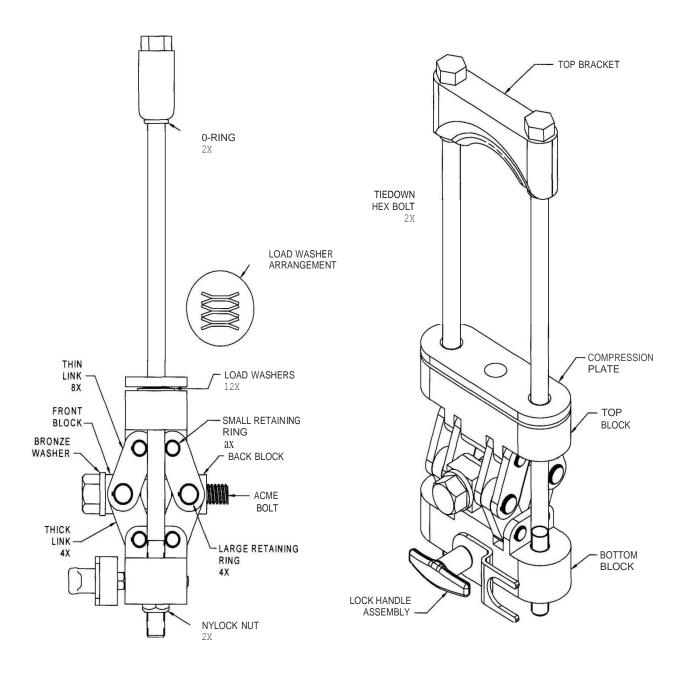
Figure 2.3-9 — Screw Jack Tiedown- Components
