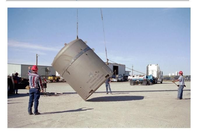
Figure 2.3-15 – TRUPACT-II Package Rotation Using Weld-On Lugs
