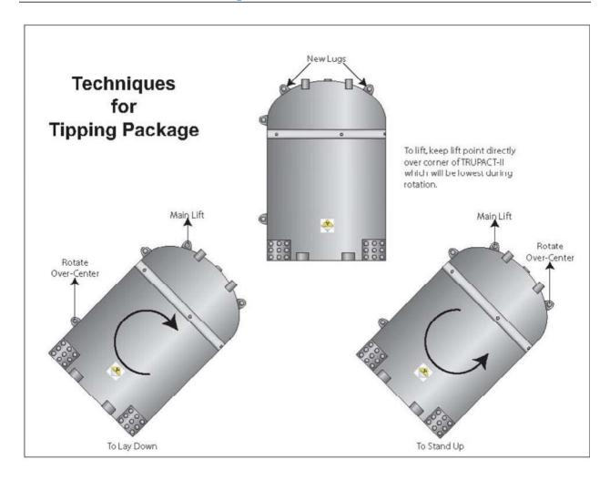
Figure 2.3-14 – Recovery Lifting Techniques for Tipping Package
