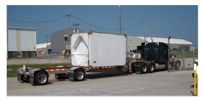
Figure 4.3.1-3 - TRUPACT-III Secured on TRUPACT-III Trailer
