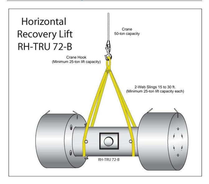
Figure 3.3-1 - Horizontal Recovery Lift RH-TRU 72-B
