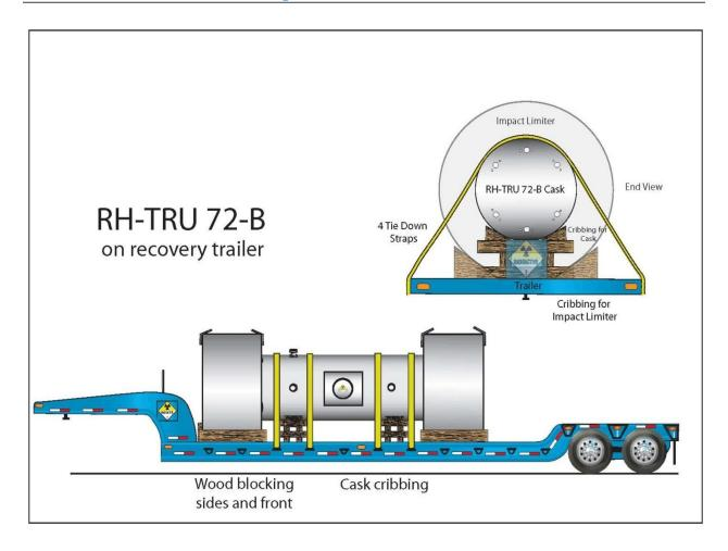
Figure 3.2-1 - RH-TRU 72-B Secured on Recovery Trailer
