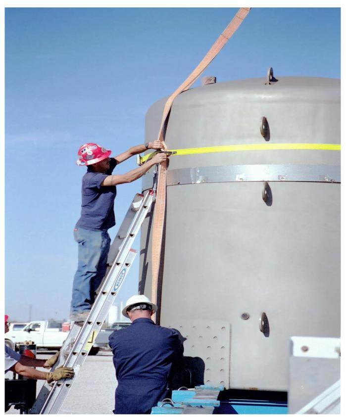
Figure 2.3-2 –Vertical Lift of a TRUPACT-II Using a Lift Sling Alignment Strap Sling is fed through the forklift pockets and up through the loops on the alignment\_strap.
