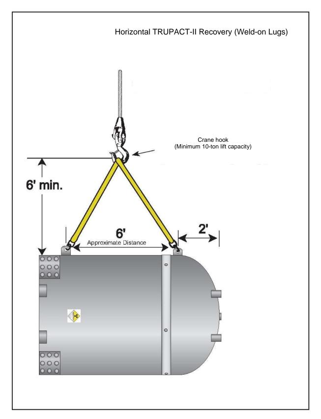
Figure 2.3-12 – Horizontal Package Lifting with Weld-On Lugs
