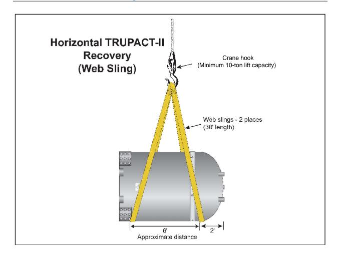
Figure 2.3-11 – Rigging for Horizontal Package Lifting (Web Sling)
