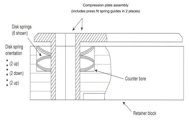
Figure 2.3-5 – Cam Handle Tiedown Assembly Disk Spring Arrangement
