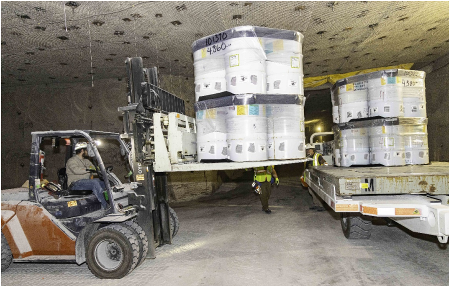
Workers offload waste drums into the underground repository's Panel 8
