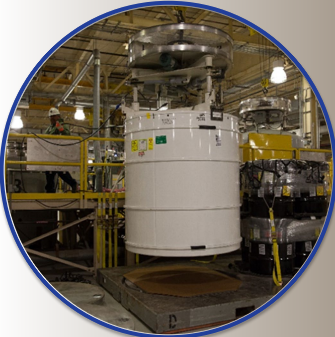
Workers unload TRU waste containers from TRUPACT-II shipping packages
