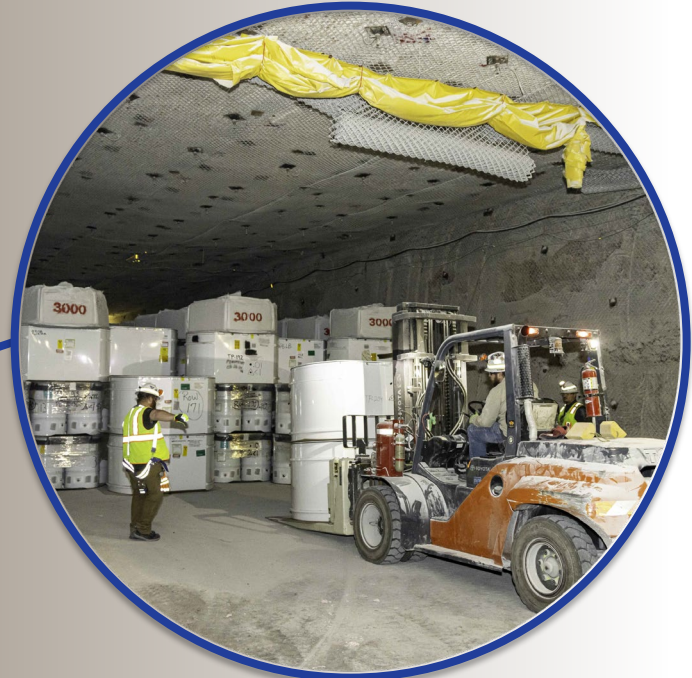
In the underground, workers systematically emplace waste drums in Panel 8 for permanent disposal
