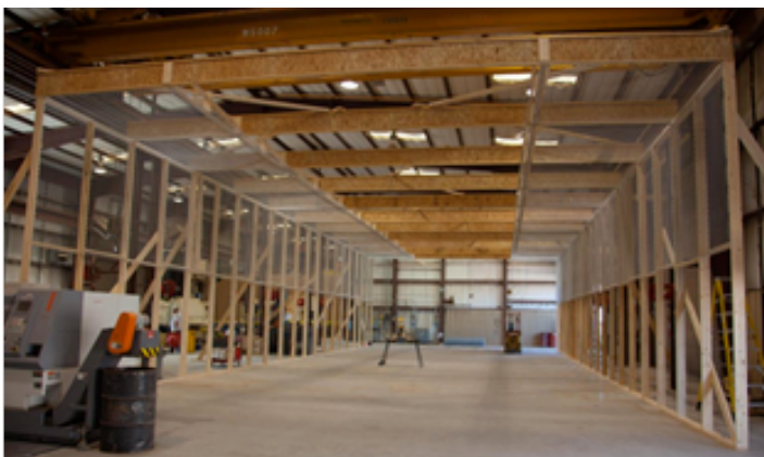
Above: WIPP has created a mock-up of Room 7 to test the various "reach" tools.
