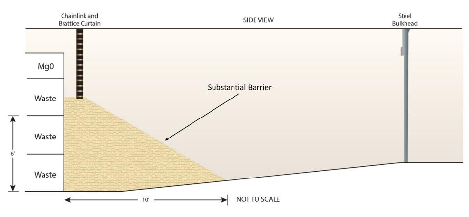
"Substantial barrier" means salt or other non-combustible material installed between the waste face and the bulkhead
