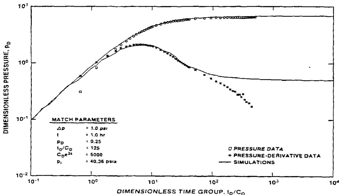
Figure 5-98. H-14/Forty-Niner Claystone Second Buildup Log-Log Plot with INTERPRET Simulation
