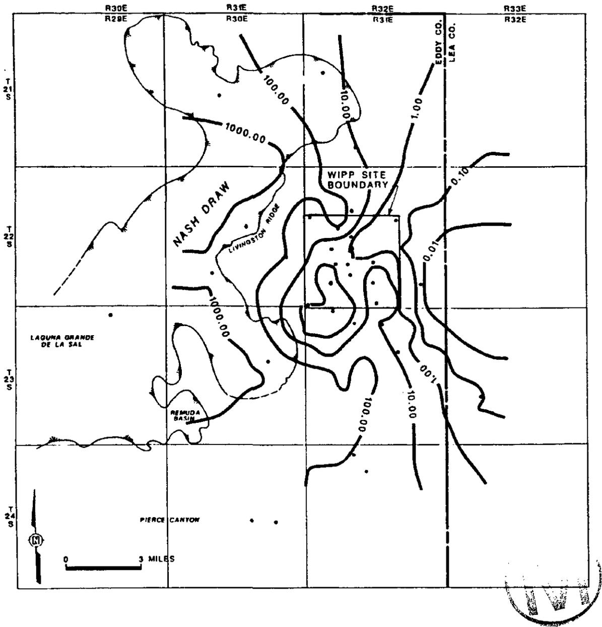
Figure 17. Calculated transmissivities for the Culebra Dolomite Member (ft<sup>2</sup>/day) (from LaVenue and others, 1988).
