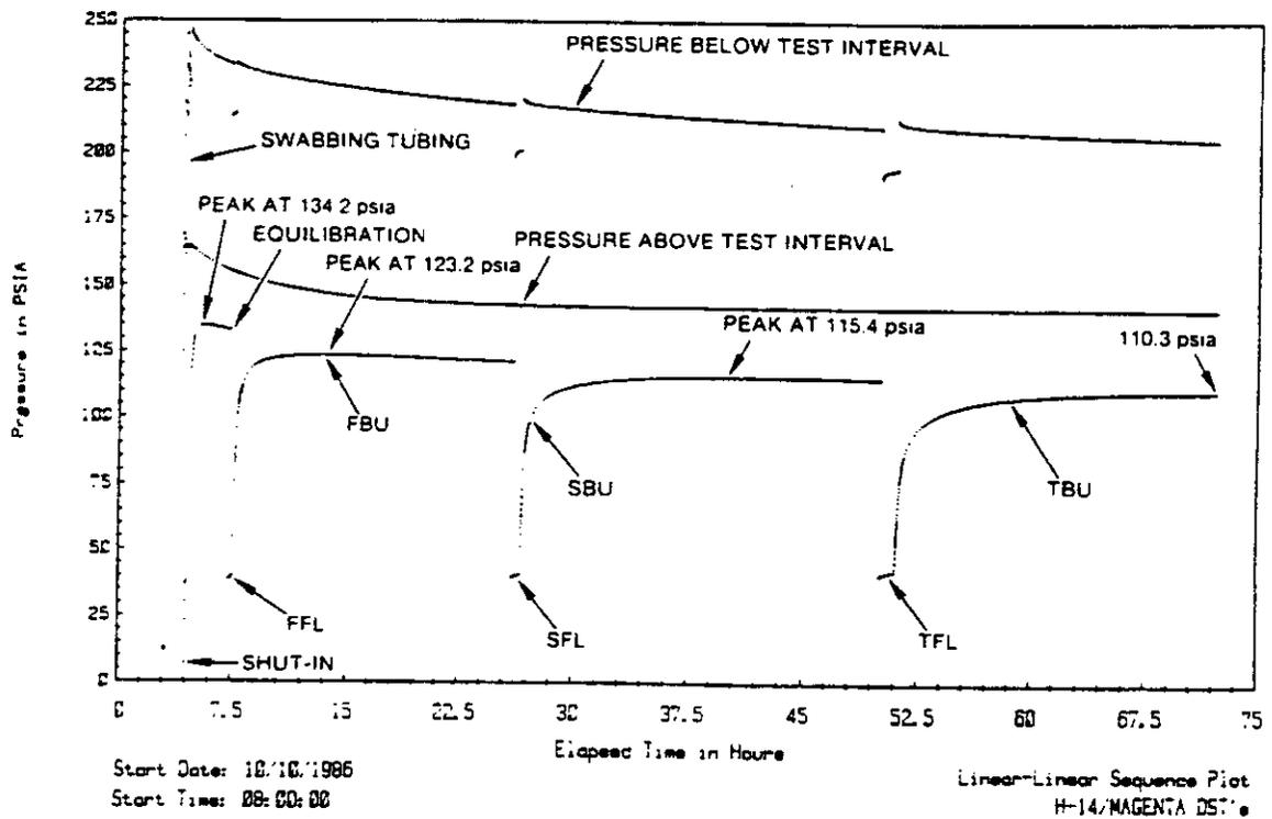
Figure 5-84. H-14/Tamarisk Claystone Shut-In Linear-Linear Sequence Plot
