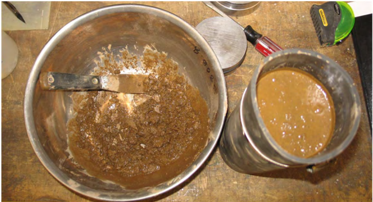
Figure 11. Batch of 100% degraded surrogate material being readied to be introduced into a Lexan sample holder.
