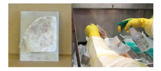
Figure 2. Salt test coupon and water washing technique used in the laboratory
