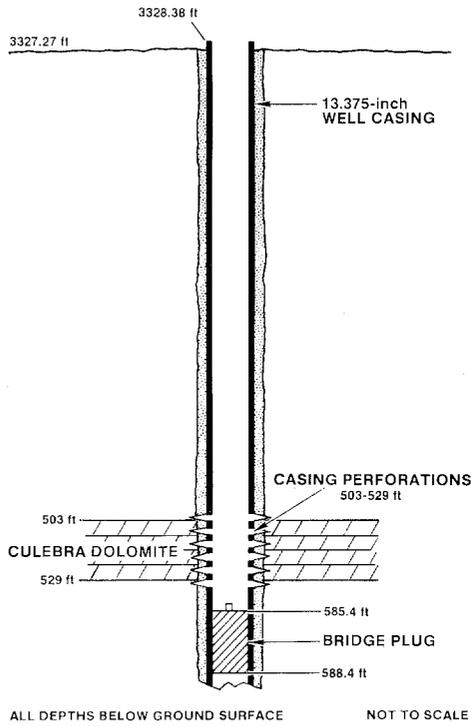
Figure 3-9. Configuration of Observation Well Cabin Baby-1.
