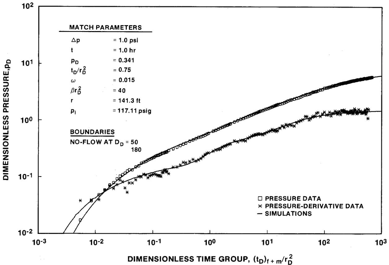
Figure 6-16. Log-Log Plot of H-11b4 Recovery During the H-11 Multipad Pumping Test.
