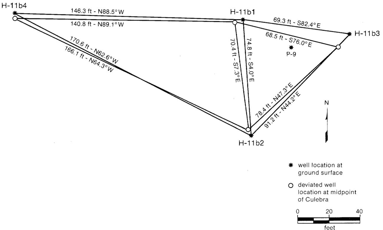
Figure 1-2. Well Locations on the H-11 Hydropad.
