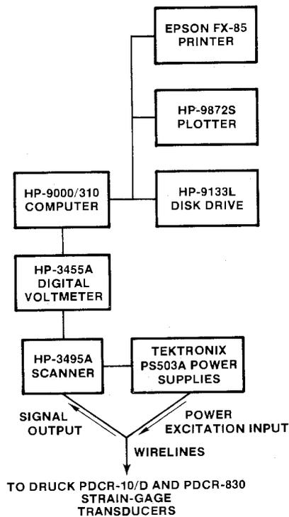
**Figure 4-6. Data-Acquisition System for the H-11b4 Pumping Test.**
