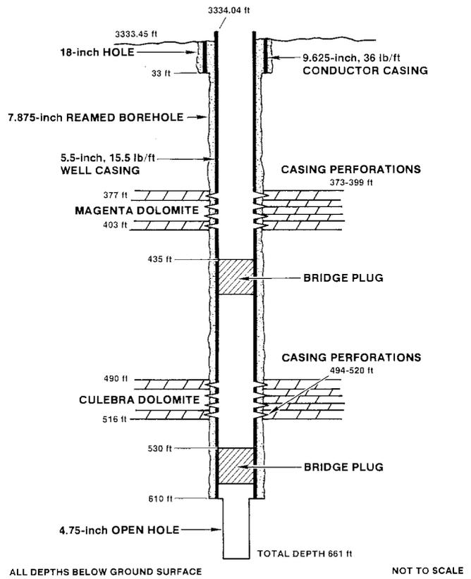
Figure 3-14. Configuration of Magenta Observation Well H-4c.
