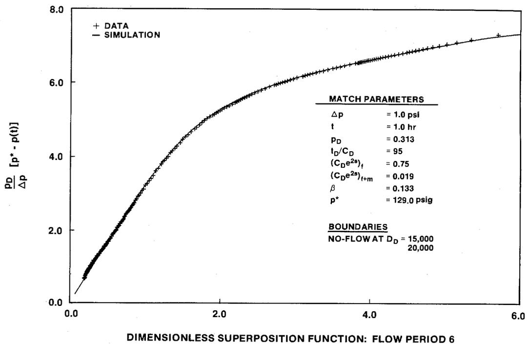
Figure 6-11. Dimensionless Horner Plot of H-11b1 Recovery During the H-11 Multipad Pumping Test.
