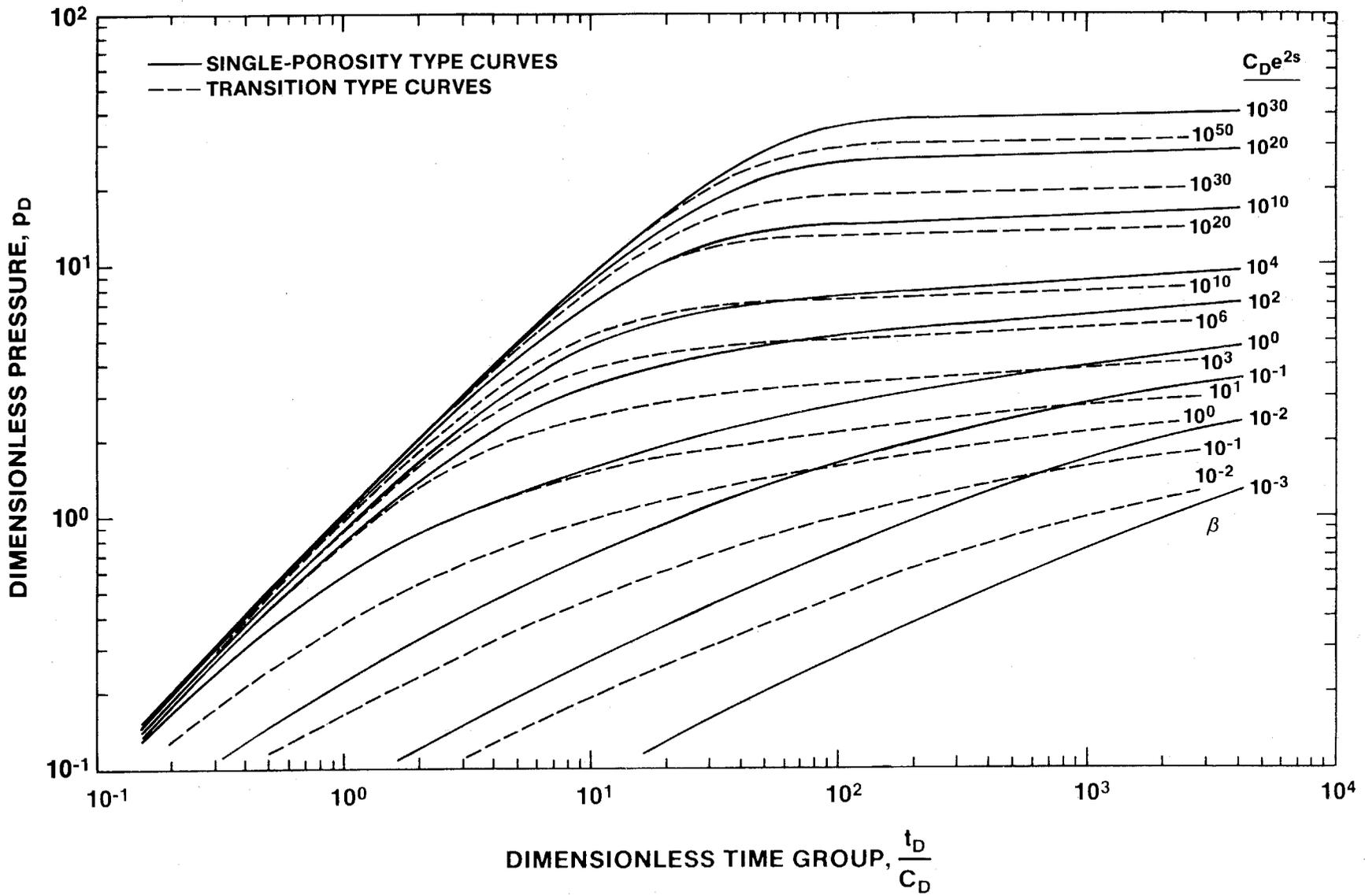
Figure B-6. Double-Porosity Type Curves for Wells with Wellbore Storage, Skin, and Unrestricted Interporosity Flow.
