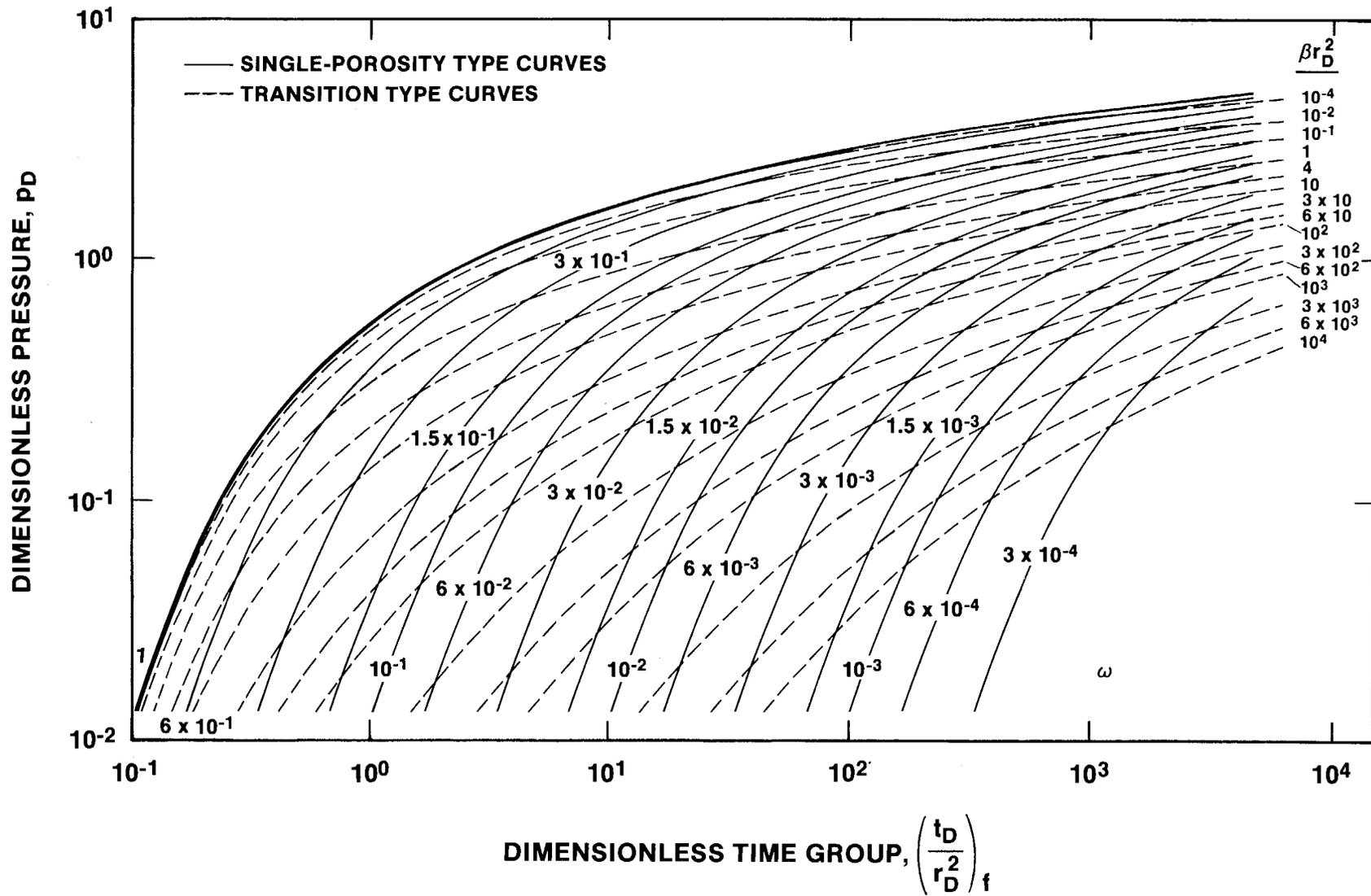
Figure B-9. Double-Porosity Line-Source-Solution Type Curves for Aquifers with Unrestricted Interporosity Flow.
