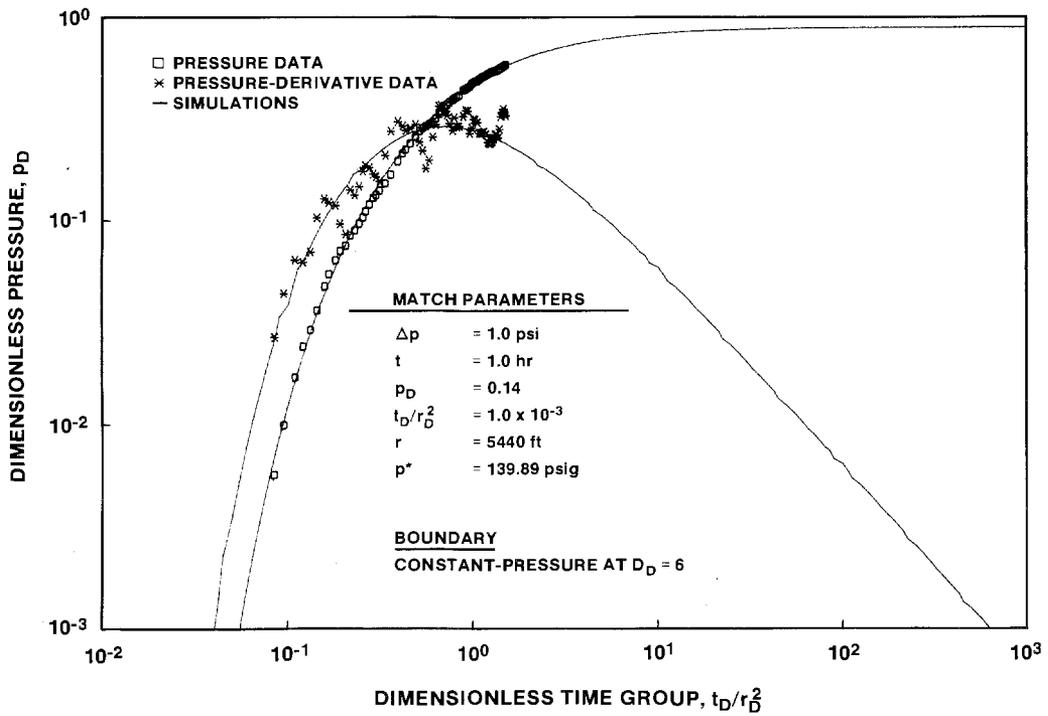
Figure 6-37. Log-Log Plot of H-17 Drawdown During the H-11 Multipad Pumping Test.
