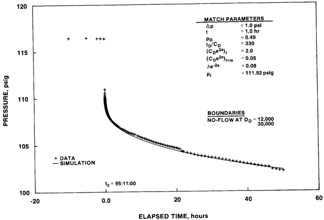
Figure 6-4. Linear-Linear Plot of H-11b4 Drawdown During the H-11b4 Pumping Test.
