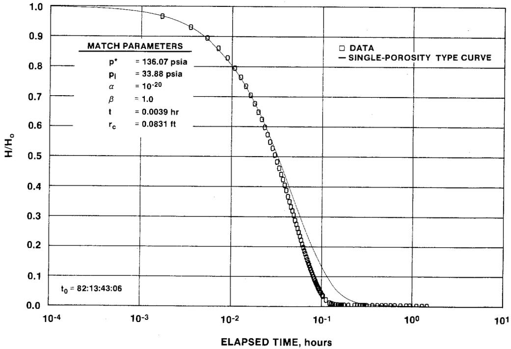
Figure 6-2. H-11b4 Slug-Test #2 Plot.
