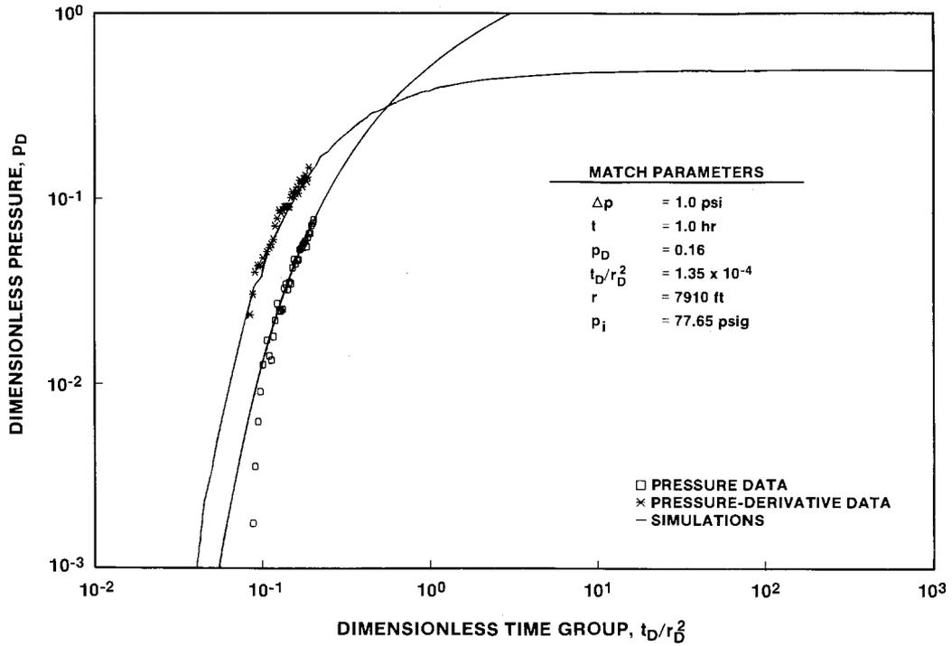
Figure 6-44. Log-Log Plot of Cabin Baby-1 Drawdown During the H-11 Multipad Pumping Test.
