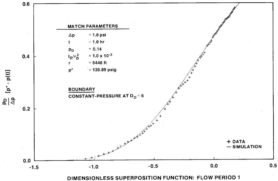
Figure 6-38. Dimensionless Horner Plot of H-17 Drawdown During the H-11 Multipad Pumping Test.
