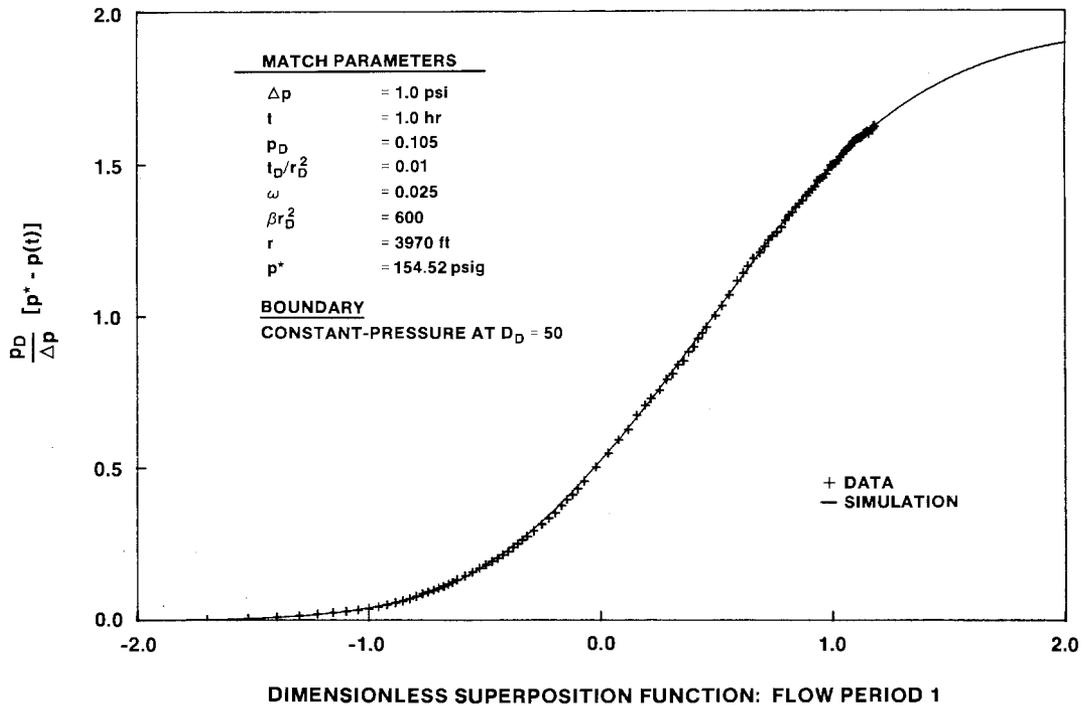
Figure 6-20. Dimensionless Horner Plot of DOE-1 Drawdown During the H-11 Multipad Pumping Test.
