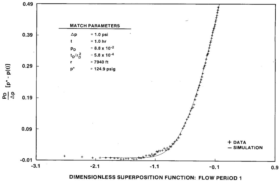
Figure 6-26. Dimensionless Horner Plot of H-3b2 Drawdown During the H-11 Multipad Pumping Test.
