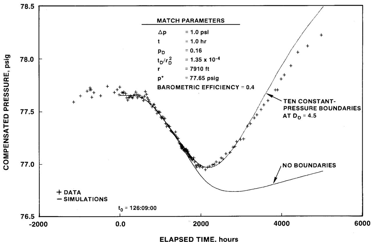
Figure 6-46. Linear-Linear Plot of Cabin Baby-1 Response During the H-11 Multipad Pumping Test.
