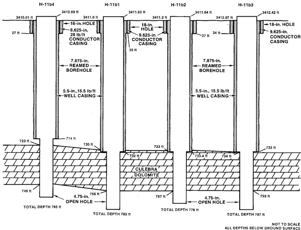
Figure 3-1. As-Built Configurations of the H-11 Wells.
