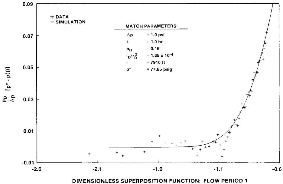
Figure 6-45. Dimensionless Horner Plot of Cabin Baby-1 Drawdown During the H-11 Multipad Pumping Test.
