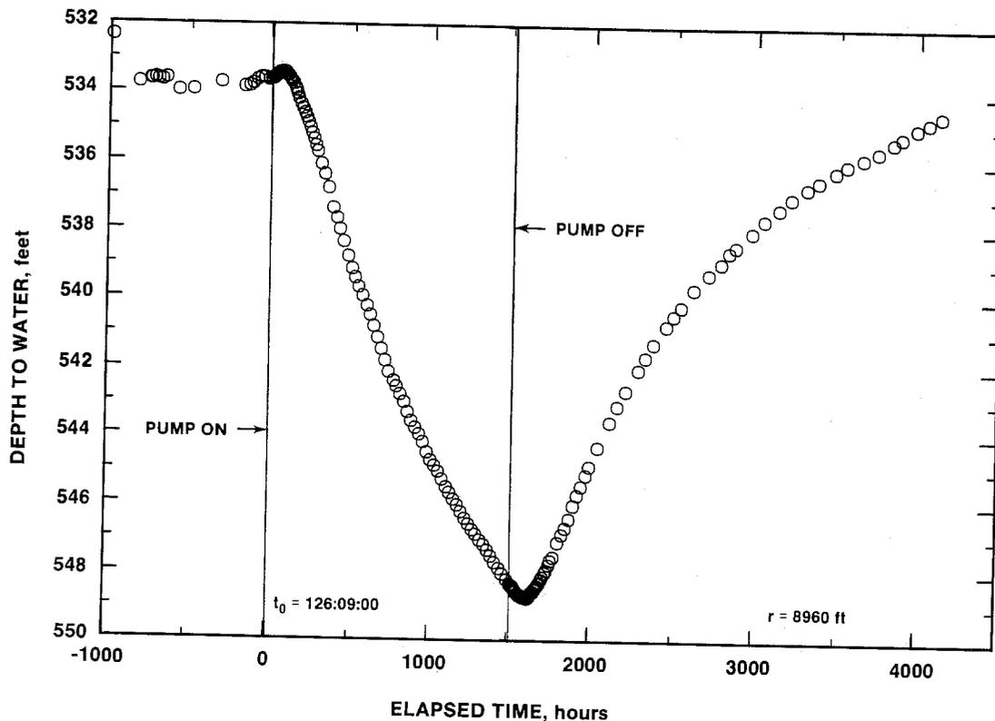
Figure 5-15. H-15 Water-Level Record During the H-11 Multipad Pumping Test.
