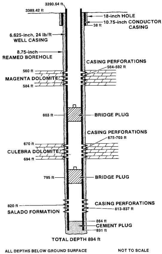
Figure 3-13. Configuration of Magenta Observation Well H-3b1.
