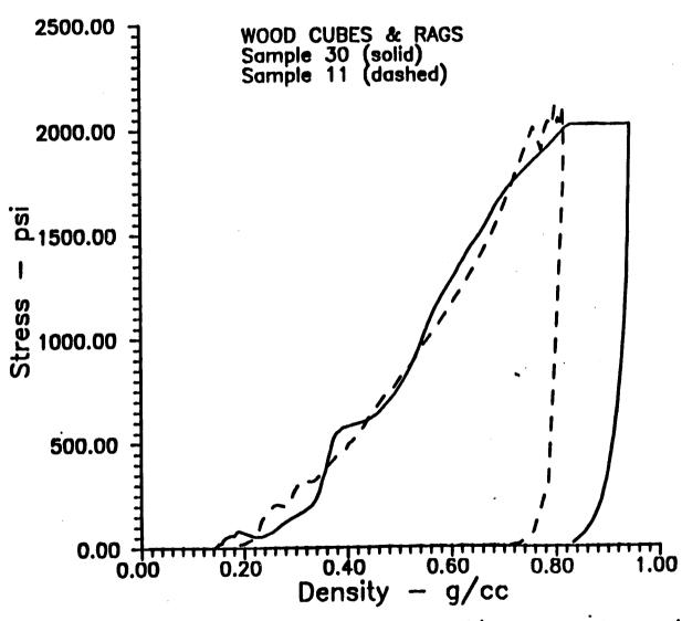
Figure 3: Stress versus density compaction curves for a mixture of wood cubes and rags simulating cellulosic waste.
