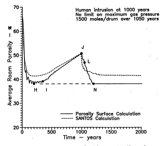
Figure 7: The average room porosity history of a disposal room as a function of time assuming that there is no limit on maximum gas pressure (Case 1).
