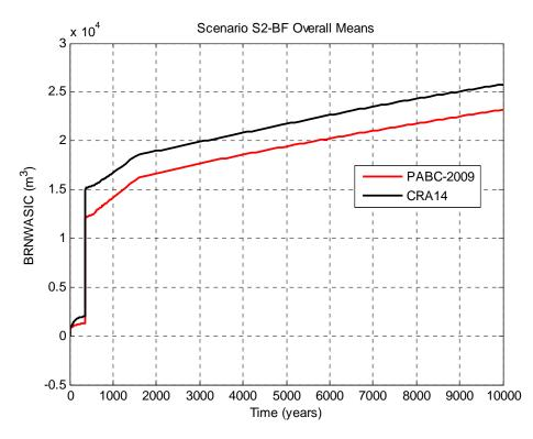
Figure 6-27: Overall Means of Cumulative Brine Inflow to the Waste Panel, Scenario S2-BF.
