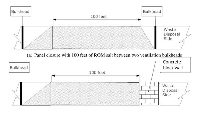
(b) Panel closure with 100 feet of ROM salt between a ventilation bulkhead & explosion wall
