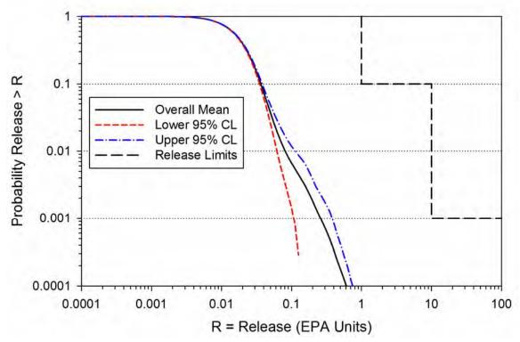
Figure 6-52: CRA-2014 PA Confidence Limits on Overall Mean for Total Normalized Releases
