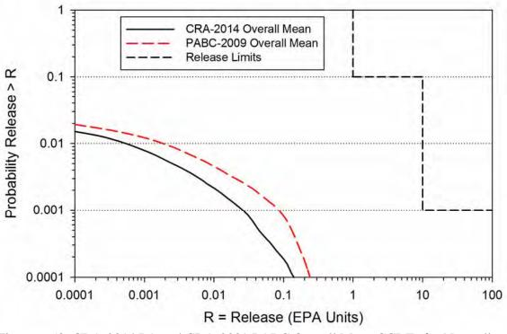
Figure 6-50: CRA-2014 PA and CRA-2009 PABC Overall Mean CCDFs for Normalized Culebra Transport Releases
