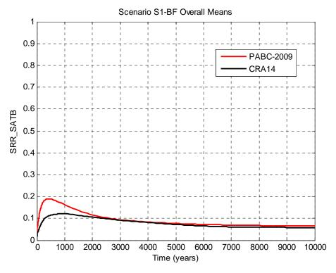
Figure 6-23: Overall Means of SRoR Saturation, Scenario S1-BF.
