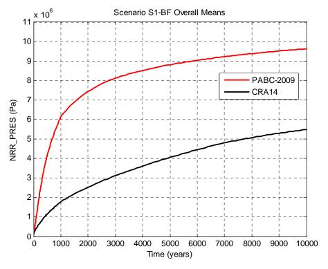
Figure 6-13: Overall Means of NRoR Pressure, Scenario S1-BF
