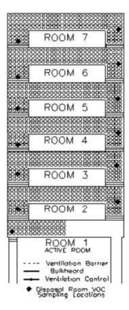
Figure 5.6 – Typical Disposal Room VOC Sampling Locations
