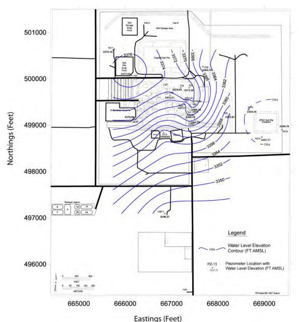
Figure 6. 17 – SSW Potentiometric Surface
