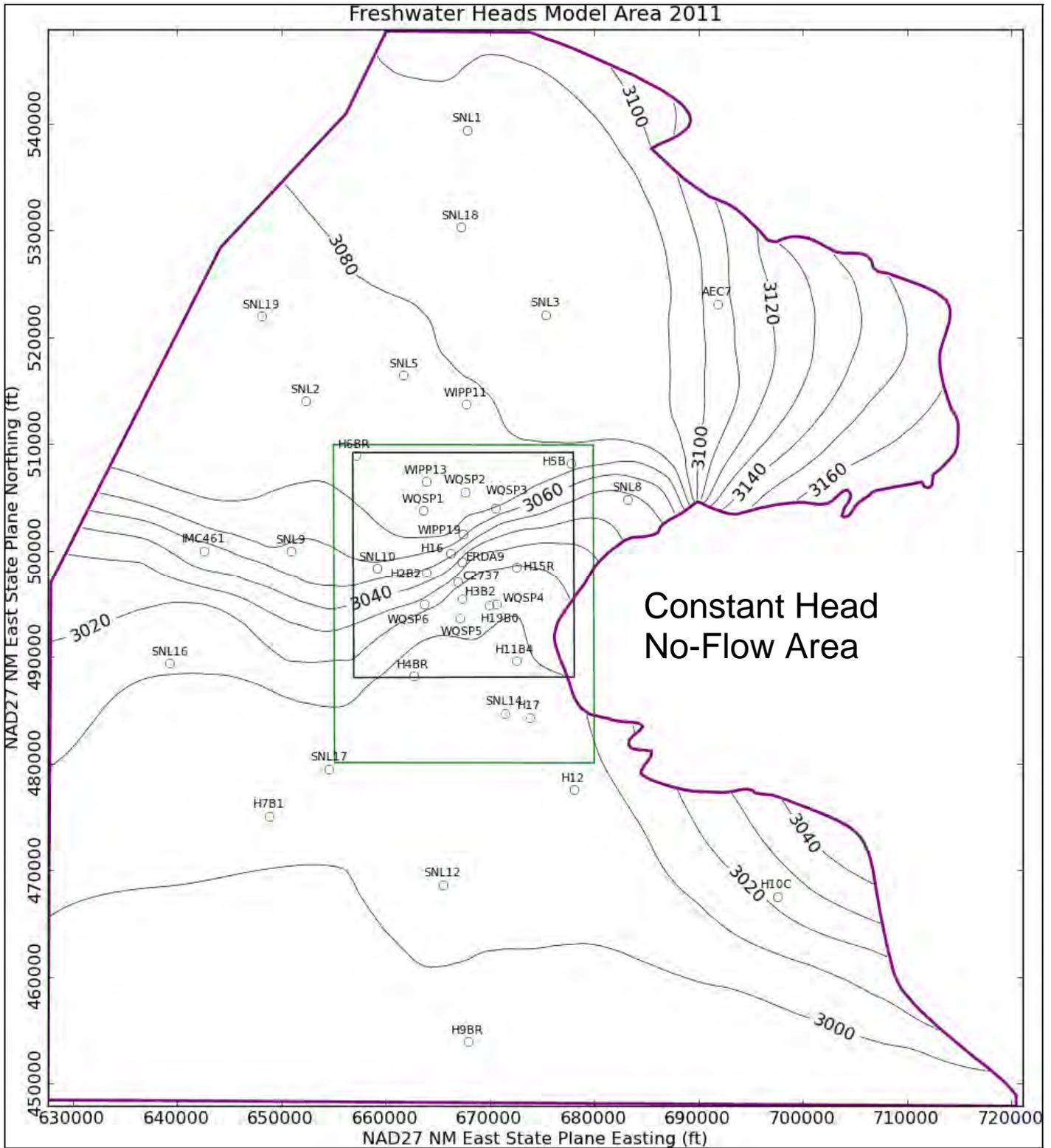
Figure 6.10 – Model Generated August 2011 Freshwater Head Contours in the Model Domain (contour interval in ft amsl)
