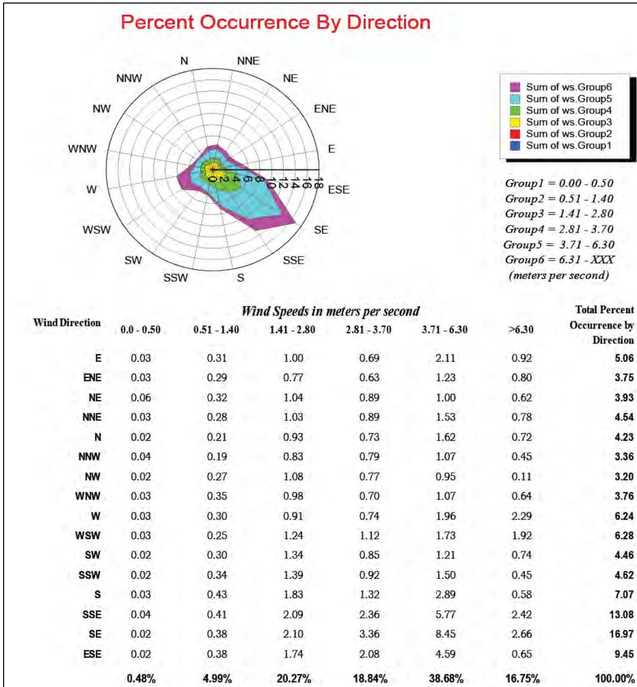
Figure 5.5 – Wind Speed (at 10-m level) Report for 2011
