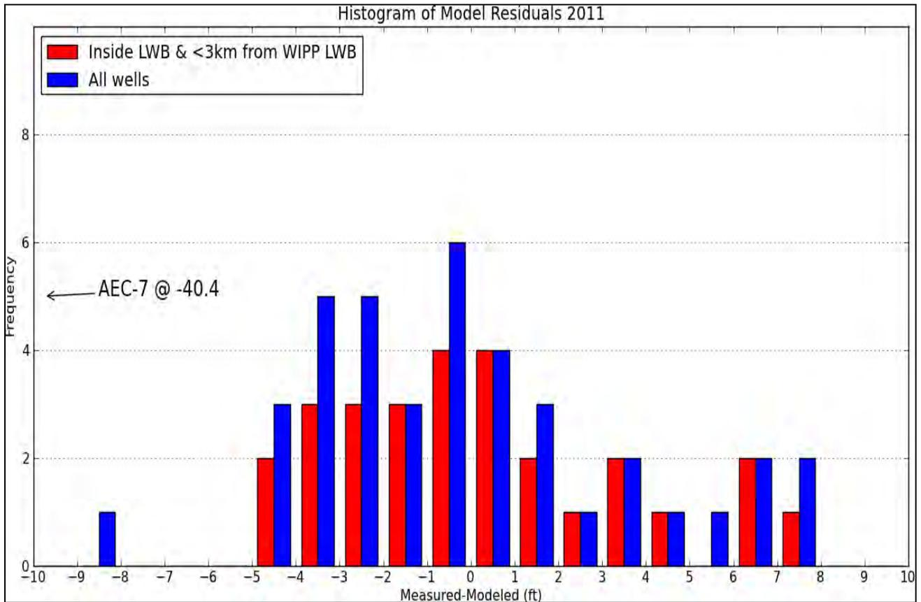
Figure 6.13 – Frequency of Modeled Freshwater Head Residuals
