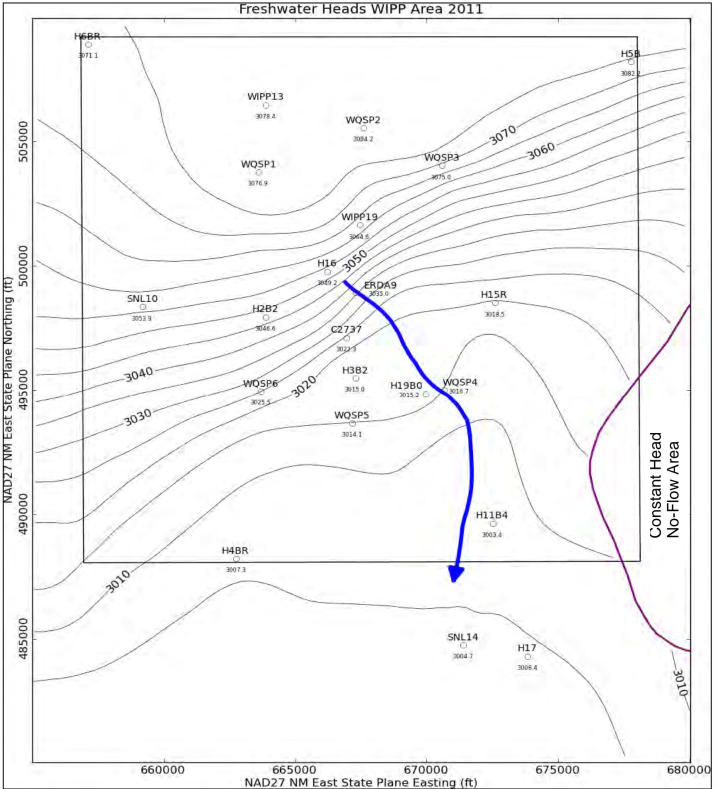
Figure 6.11 – Model-generated August 2011 Freshwater Head Contours (5-foot Contour Interval) in the WIPP Vicinity with Blue Water Particle Track from Waste Handling Shaft to WIPP Land Withdrawal Boundary (contour interval in ft amsl)
