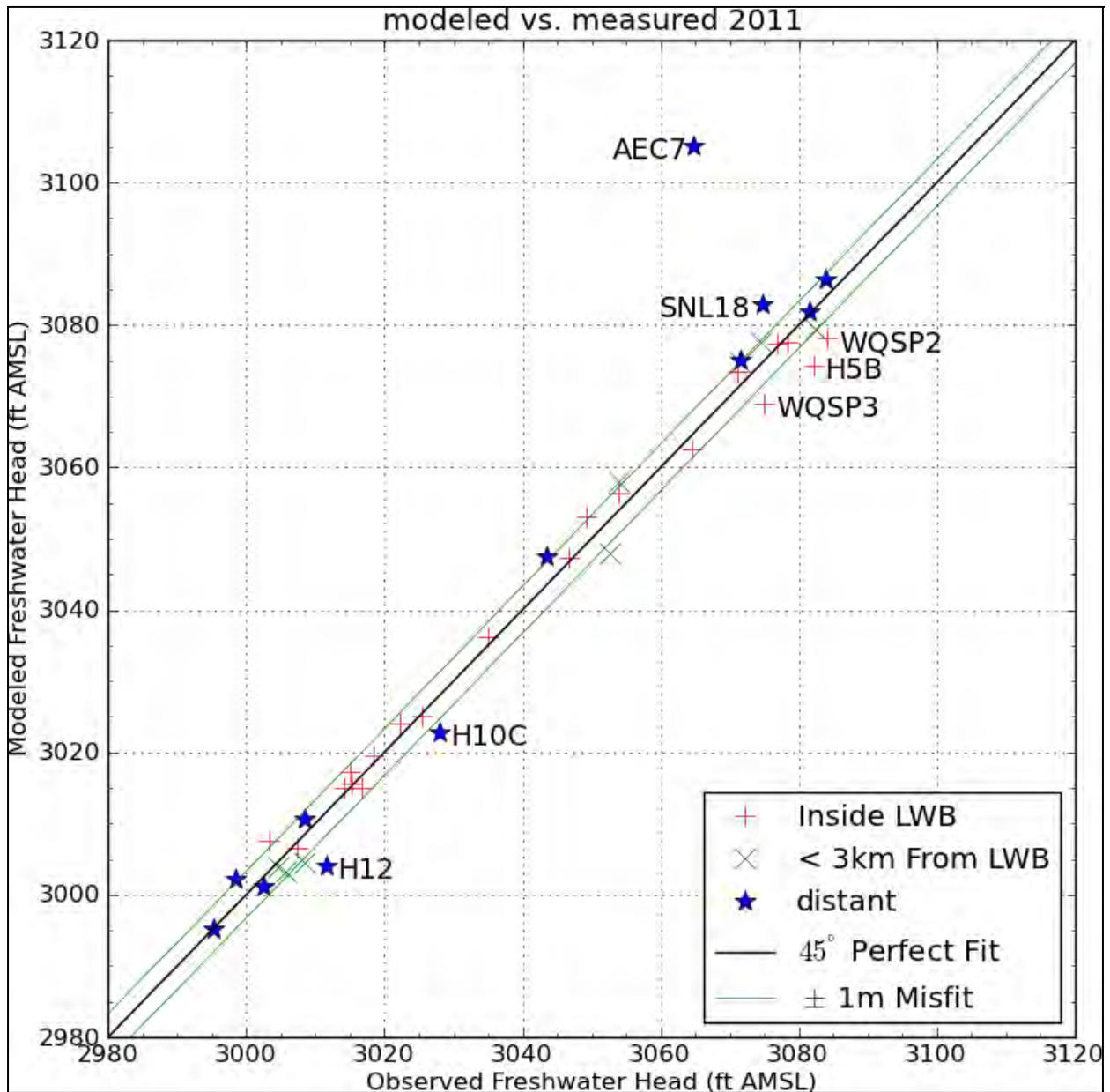
Figure 6.12 – Measured Versus Modeled Scatter Plot for PEST-calibrated MODFLOW 2000 Generated Heads and August 2011 Observed Freshwater Heads
