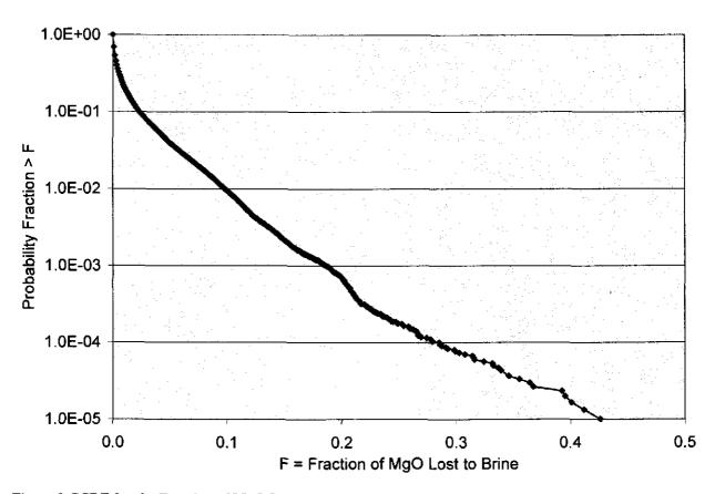
Figure 2 CCDF for the Fraction of MgO Lost to Brine Outflow
