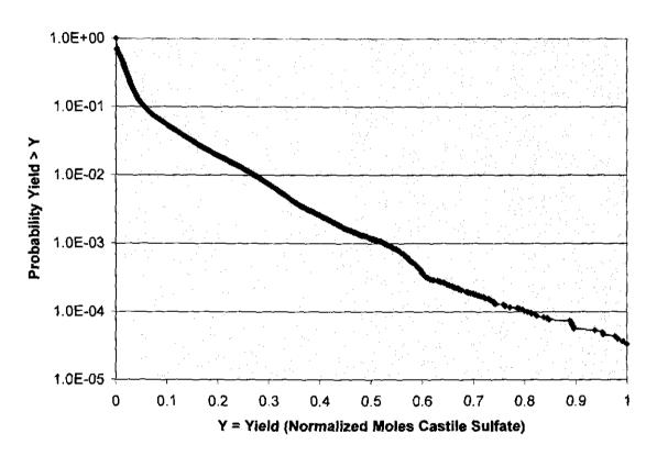
Figure 1 CCDF of Normalized Moles of Castile Sulfate that enter the "Worst Case" Waste Panel (Figure 1 from Clayton and Nemer (2006))
