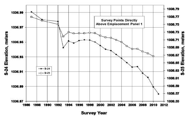
Figure 2.3. Elevations of WIPP monuments S-24 and S-25 located directly above emplacement Panel 1.
