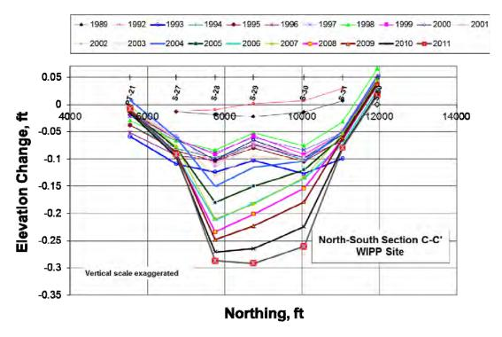
Figure 2.10. East-West subsidence profile C-C'.
