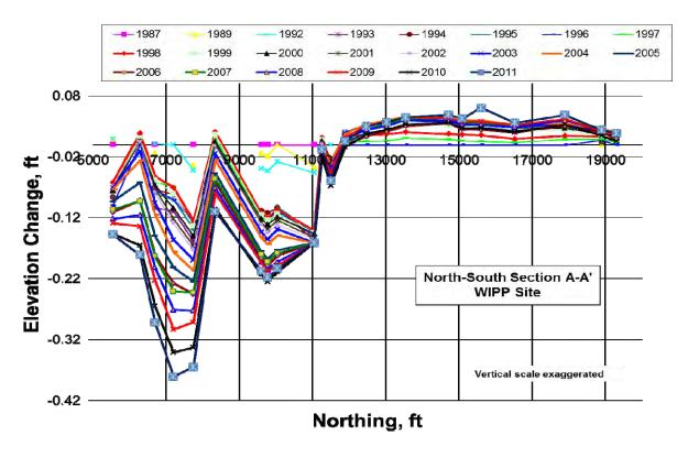
Figure 2.8. North-South subsidence profile A-A'.
