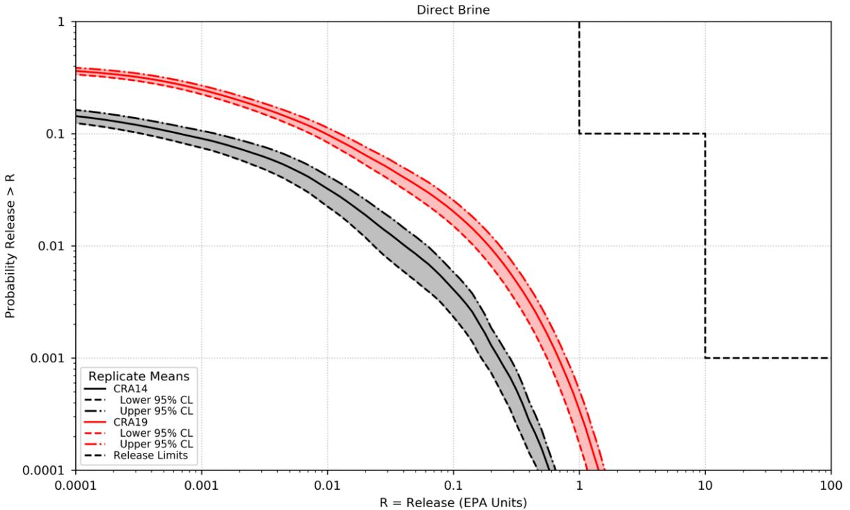
Figure 14 – Confidence Limits on Overall Mean for Normalized Direct Brine Releases
