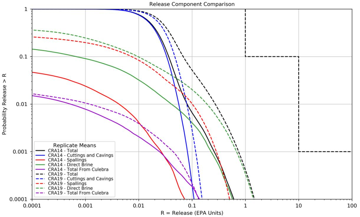
**Figure 25 – Comparison of Overall Means for Release Components**
