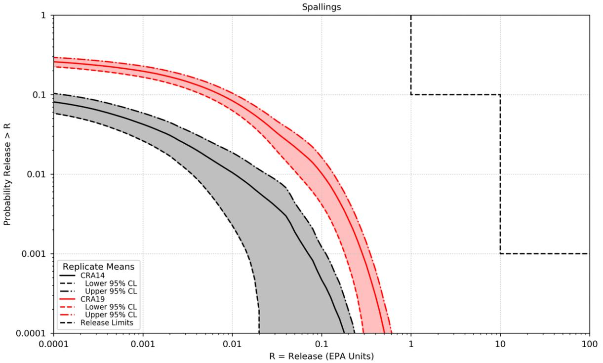
**Figure 9 – Confidence Limits on Overall Mean for Normalized Spallings Releases**
