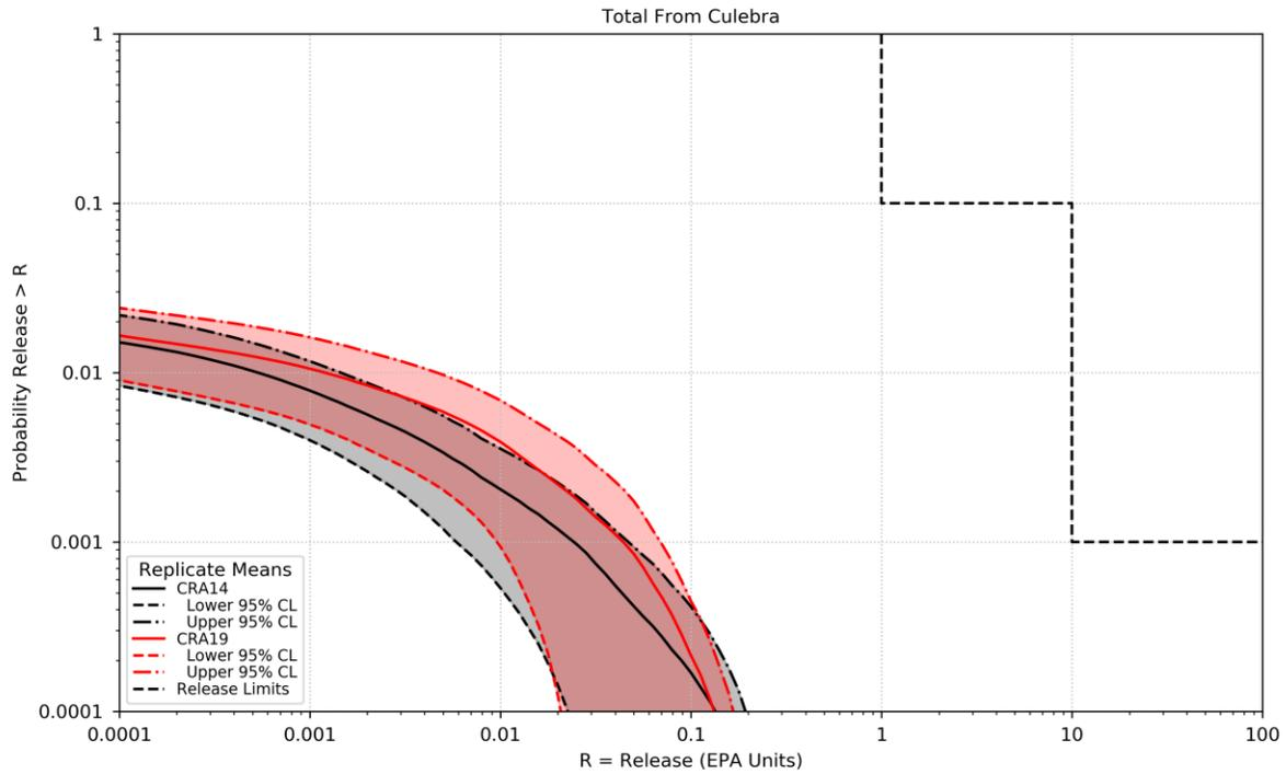
**Figure 20 – Confidence Limits on Overall Means for Transport Releases from the Culebra**
