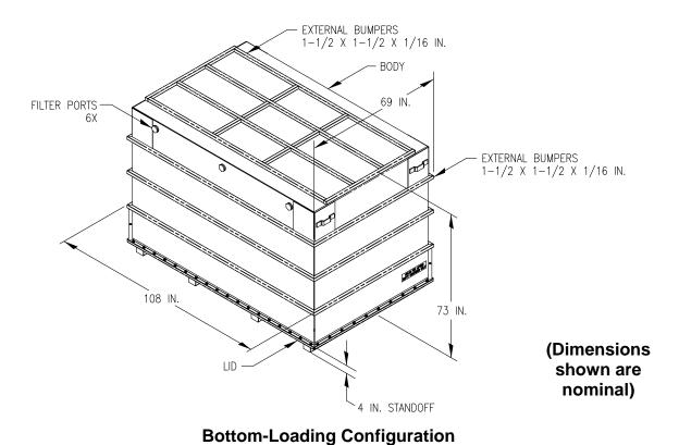
Figure 2.8-1 – Schematic of SLB2
