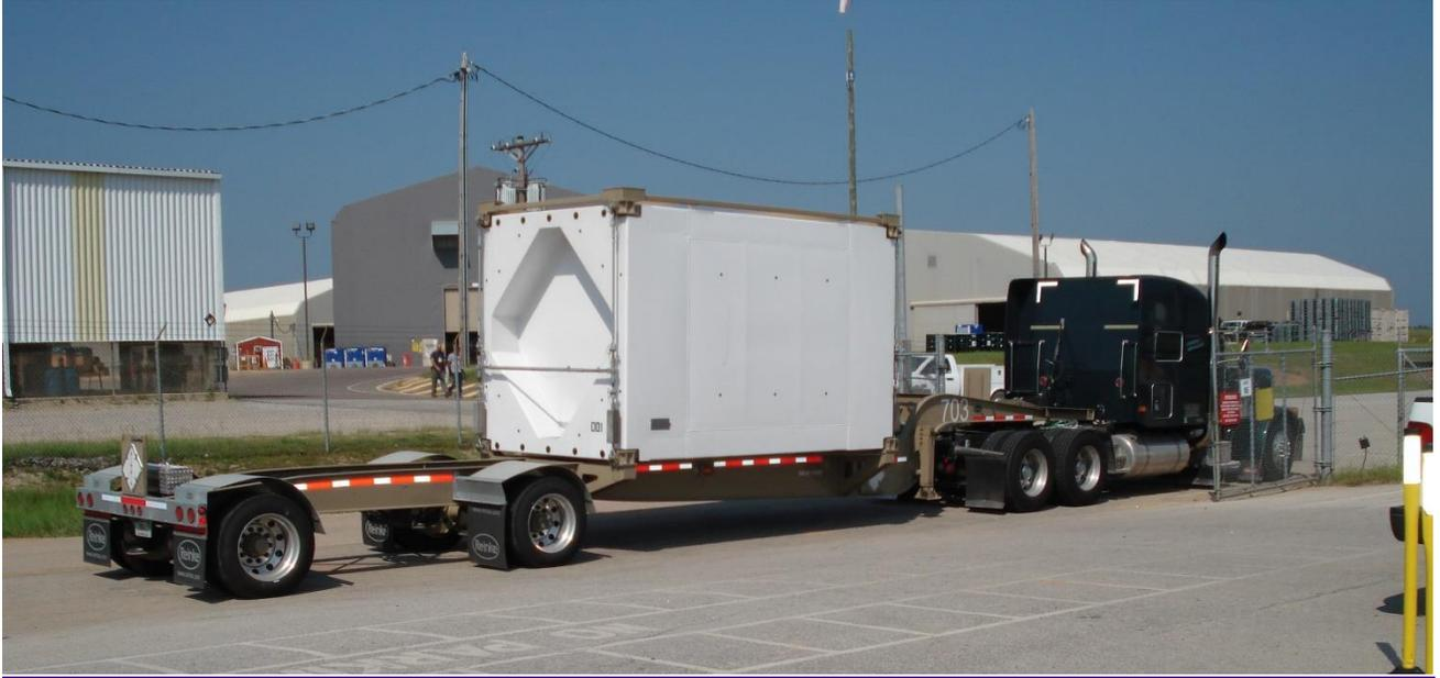
**Figure 4.3.1-3 – TRUPACT-III Secured on TRUPACT-III Trailer**
