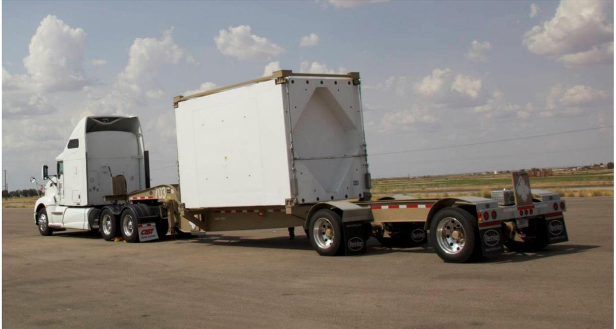
**Figure 4.3.2-1 – TRUPACT-III on a Trailer Secured by ISO Container lugs on bottom corners**
