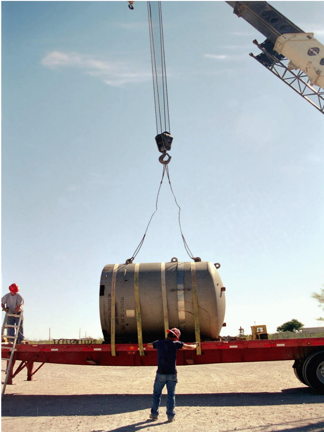
Figure 2.3-13 – Horizontal Lift and Securement of a TRUPACT-II Using Weld-On Lugs
