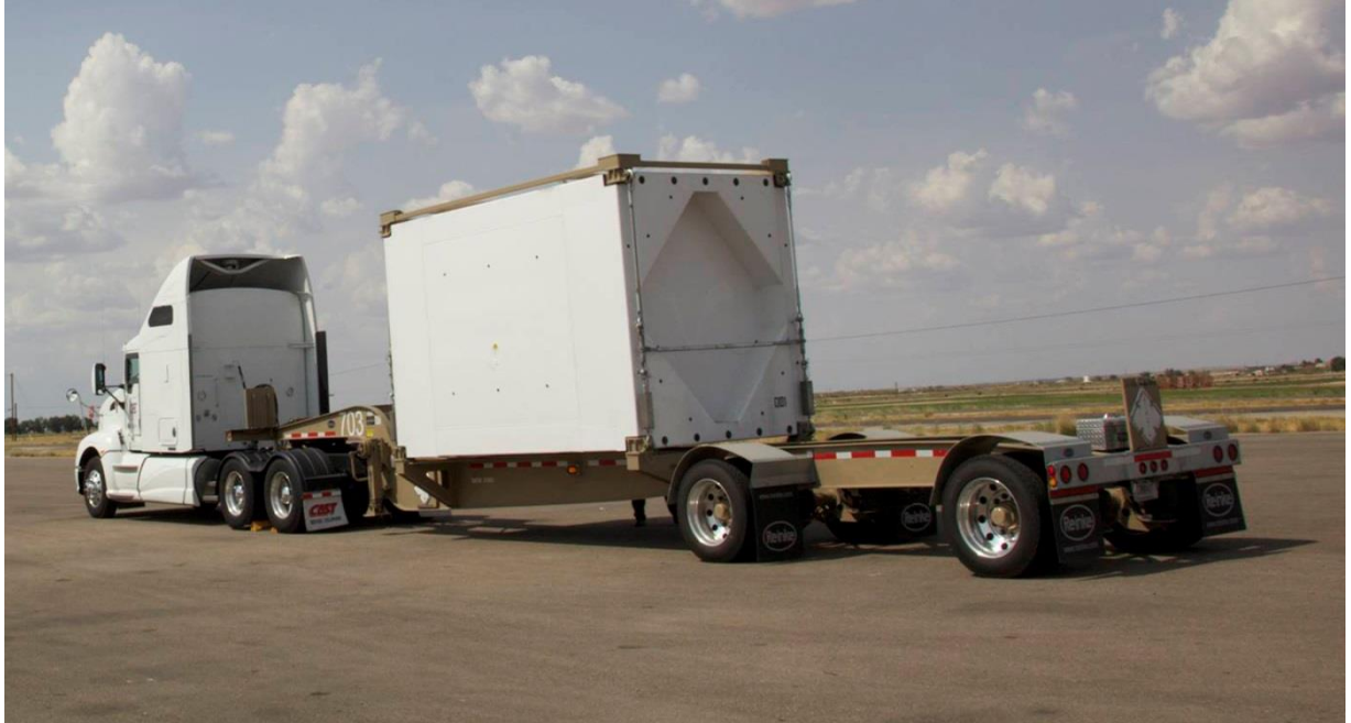
Figure 4.3.2-1 TRUPACT-III on a Trailer Secured by ISO Container lugs on bottom corners.
