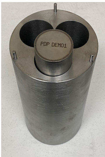
Figure F-3. Cut Away View and Actual Source Insert Fixture Assembly (Insert Fixture with Cover Ring and Demonstration Source)
