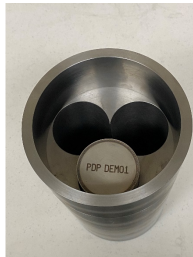
Figure F-3. Cut Away View and Actual Source Insert Fixture Assembly (Insert Fixture with Cover Ring and Demonstration Source)
