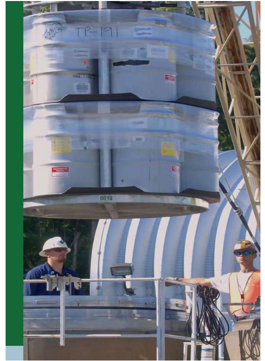
Waste containers are loaded into a TRUPACT-II shipping package
